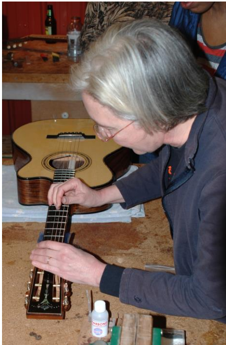
Figure 2 Temporary Nut Slot Repair
