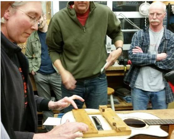
*Figure 5 Saddle Slot Cutting Jig*
