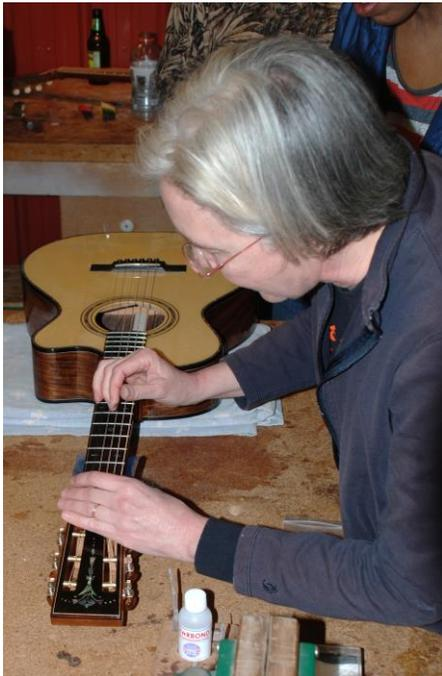
Figure 2 Temporary Nut Slot Repair
